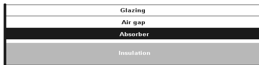
Figure 3: schematic view of the elements in a conventional collector.
